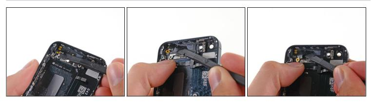
• Starting under the cable connection, use the flat of a spudger to pry the Wi-Fi antenna up from the rear case.
