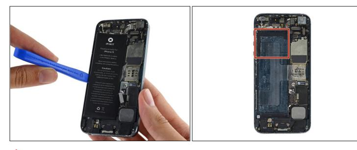
Use the plastic opening tool to gently pry the battery up, only at the outside edge of the phone. Prying anywhere else, especially near the logic board, may result in damage to the logic board.
