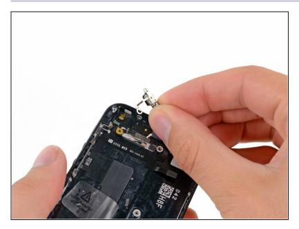
• Remove the vibrator bracket and motor from the rear case.
