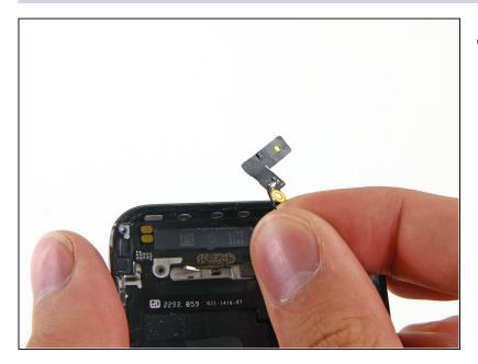
• Remove the Wi-Fi antenna from the rear case.
