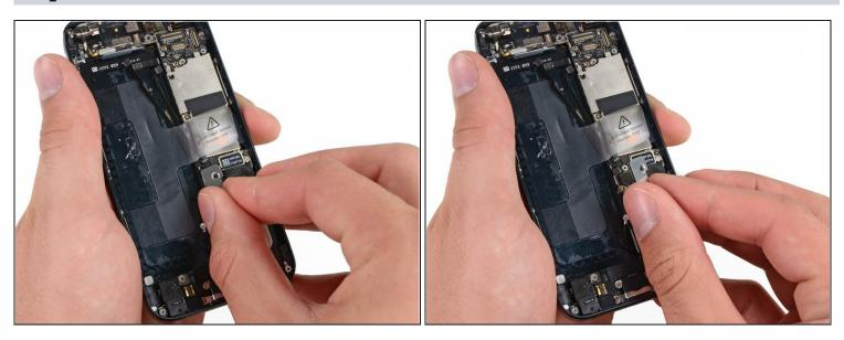
• Remove the mid-section bracket from the logic board.
