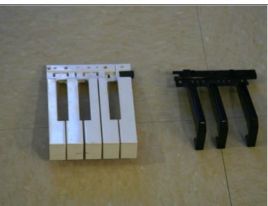
Press the tab on the back side of the block of keys out and detach the black keys.
