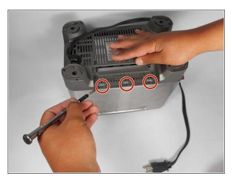
Remove the three 8mm screws using the Tri-point Y1 screwdriver.
