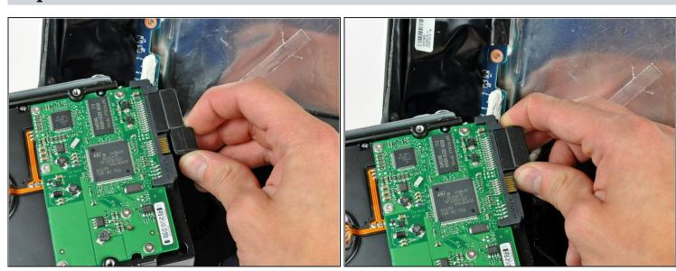
Pull both the SATA power and data cable connectors away from the hard drive.
