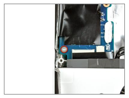
Remove the single T10 Torx screw securing the inverter board to the rear case.
