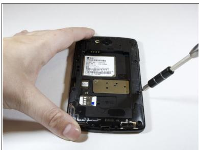
Remove the eight 4 mm screws on the inner panel using the phillips #000 Screwdriver
