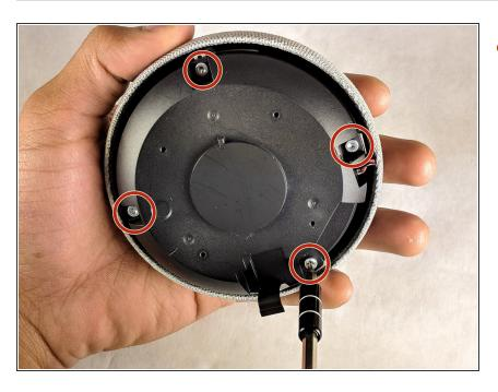
Remove the four 7.8mm T8 Torx screws.
