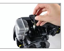
Tug the Spark Plug Cap from the top of the Spark Plug (between the OHV housing and the exhaust manifold) with your hands to remove it.
