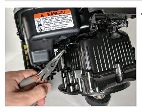
Carefully re-hook the spring on the arm it was disconnected from.
