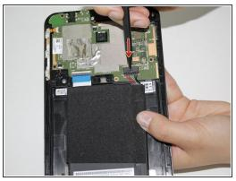
• Using the spudger, gently press on the black button on the plug port to release the battery from the plug.
