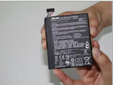
Remove the battery from the device.
