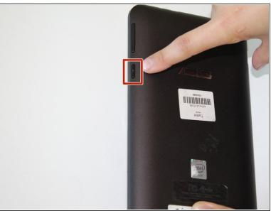
Flip over the tablet so the back cover is facing you. Hold the second button on the left below the volume buttons down until it powers off.
