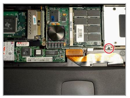
Unscrew, but do not remove, the single Phillips screw from the hard drive bracket.
