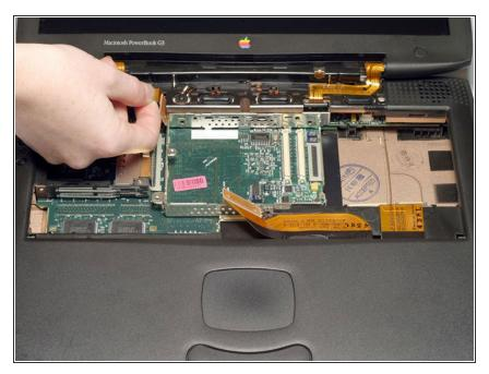
• Disconnect the orange display data cable on the left side of the computer. Grasp the cable near the connector and pull directly up.
