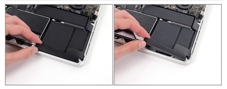
• Lift and remove the left speaker out of the upper case.
