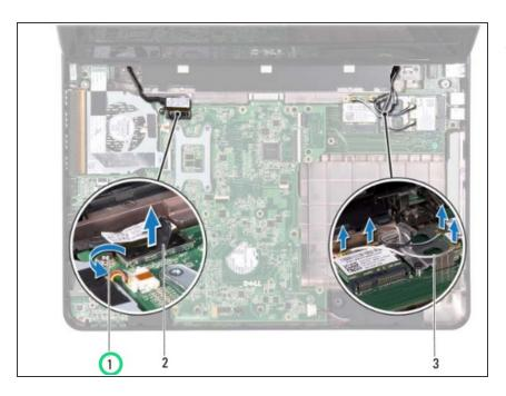
Tighten the display cable grounding screw.
