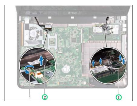
Route the display cable and Mini-Card antenna cables through the routing guides.
