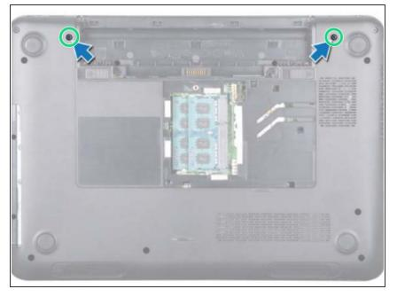
Replace the two screws at the bottom of the computer.
