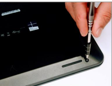
Remove the 8 screws that hold down the back panel using the Phillips #000 screwdriver.
