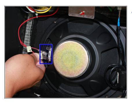
Remove the two female connection terminals from the speaker terminals.
