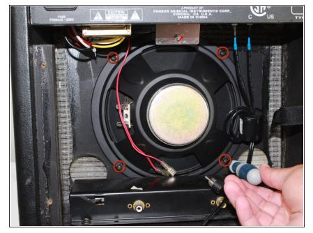
Use a Philips #1 screwdriver to remove the four 21.9 mm Phillips screws from the perimeter of the speaker.
