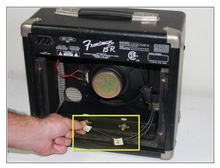
Using tape or a post-it, label the input and output wires on the reverb.
