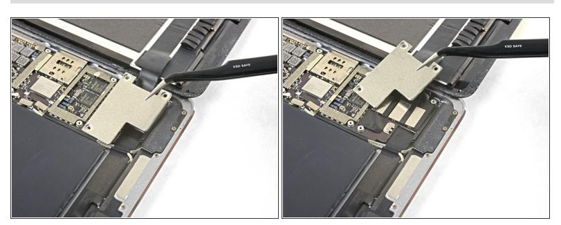
Remove the display cable bracket.
