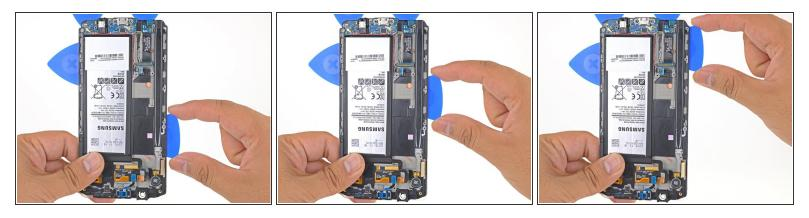
• The non-battery-edge contains a wider swath of adhesive than the other sides. Insert the opening pick as deep as you can to cut through all of it.
