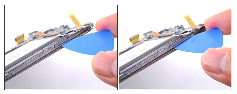
Insert an opening pick between the plastic frame and the display assembly on the same edge you
