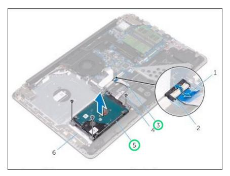
Lift the hard-drive assembly along with its cable off the palm rest and keyboard assembly.
