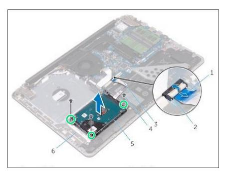
Align the screw holes on the harddrive assembly with the screw holes on the palm rest and keyboard assembly.
