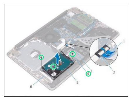
Replace the screws that secure the hard-drive assembly to the palm rest and keyboard assembly.
