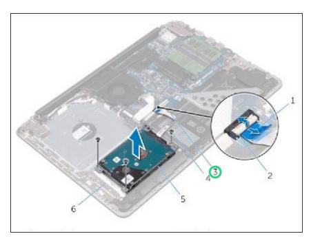
Connect the hard-drive cable to the system board and close the latch to secure the cable.
