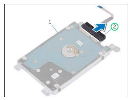
Connect the interposer to the harddrive assembly.
