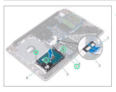
Remove the screws that secure the hard-drive assembly to the palm rest and keyboard assembly.
