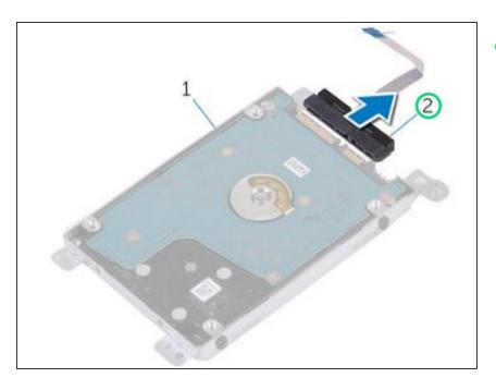
Disconnect the interposer from the hard-drive assembly.
