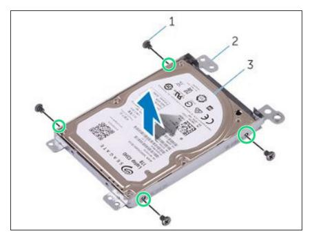
Align the screw holes on the harddrive bracket with the screw holes on the hard drive.
