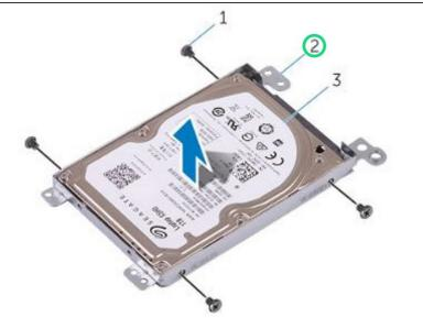
Lift the hard drive off the hard-drive bracket.
