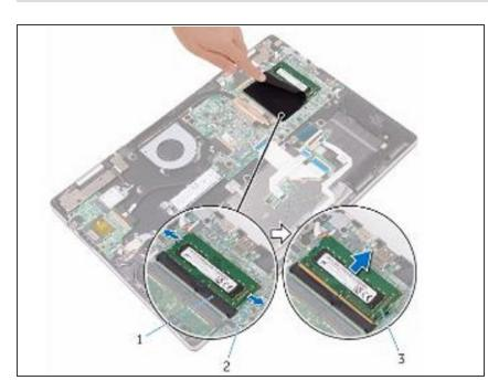
• Lift the Mylar to access the memorymodule slot.
