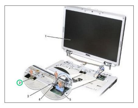
Connect the camera/microphone cable to the camera/microphone cable connector on the system board.
