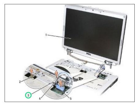
Loosen the captive grounding screw, then disconnect the display cable from the display cable connector on the system board.
