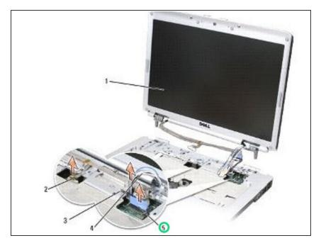
Connect the display cable to the display cable connector on the system board.
