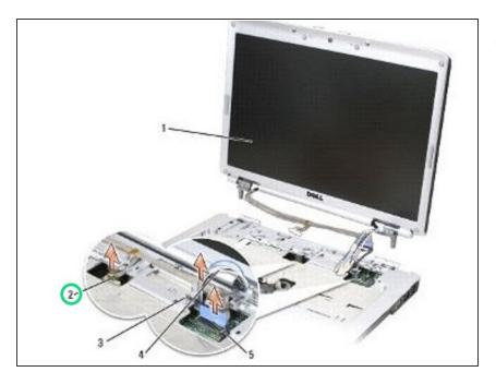
Disconnect the camera/microphone cable from the camera/microphone cable connector on the system board.
