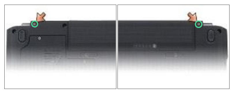
Replace the two M2.5 x 8-mm screws on the bottom of the computer.
