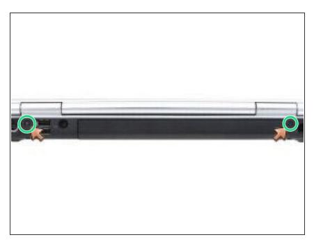
Replace the two M2.5 x 8-mm screws on the back of the computer.
