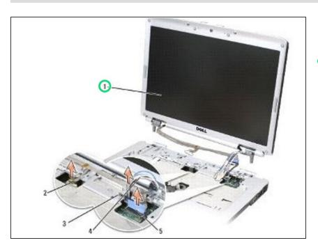
Lift the display assembly out of the computer.
