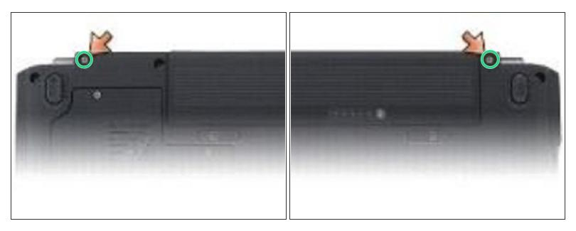
Remove the two M2.5 x 8-mm screws from the bottom of the computer.
