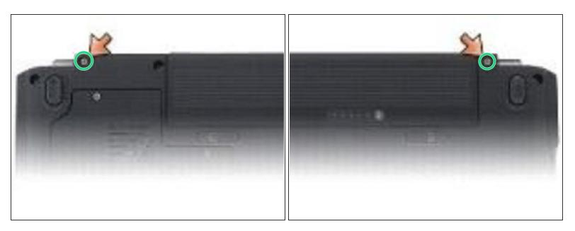
Loosen the two captive screws that secure the Mini Card compartment cover, then remove the cover and set it aside.
