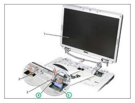
Route the display cable and antenna cables beneath the plastic tabs on the palm rest.
