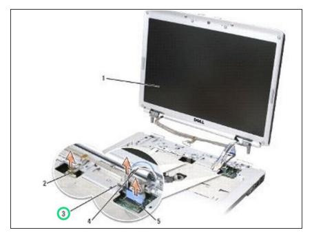
Replace and tighten the captive grounding screw.
