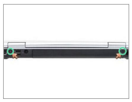
Remove the two M2.5 x 8-mm screws from the back of the computer.
