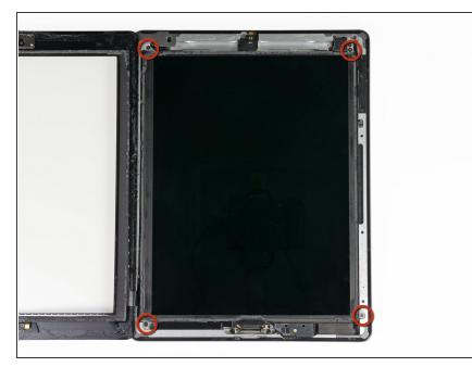
Remove the four 2 mm Phillips #00 screws securing the LCD to the aluminum frame.
