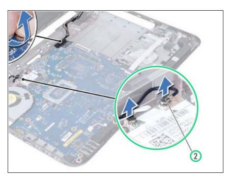
Disconnect the wireless mini-card cables from the connectors on the wireless mini-card.
