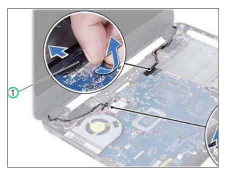
• Disconnect the display cable from the connectors on the system board.
