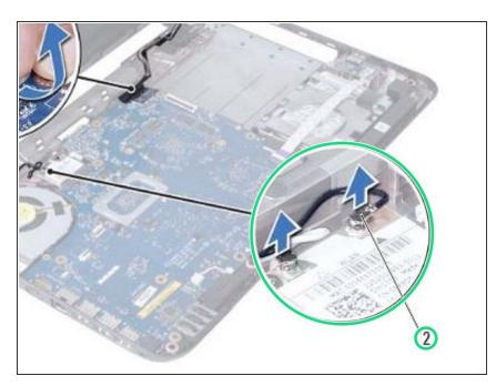
Connect the wireless mini-card cables to the connectors on the wireless mini-card.
