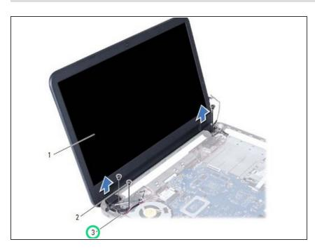
• Move aside the power adapter-port cable from the screws.
