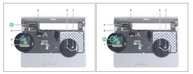
• Disconnect the display cable and remove the screw from the system board.
