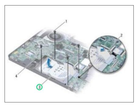
Slide and lift the hard drive assembly out of the computer base.
