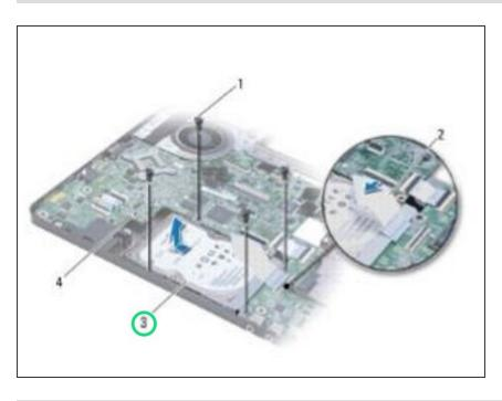
Slide the hard drive assembly into the computer base until it is fully seated.
