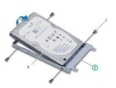
• Place the **NEW** hard drive in the hard drive bracket and replace the four screws that secure the hard drive bracket to the hard drive.
