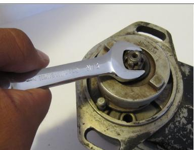
Use a 9/16 wrench to unscrew the nut on the drive shaft.
