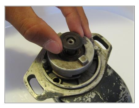
Remove the lock washer underneath the nut.
