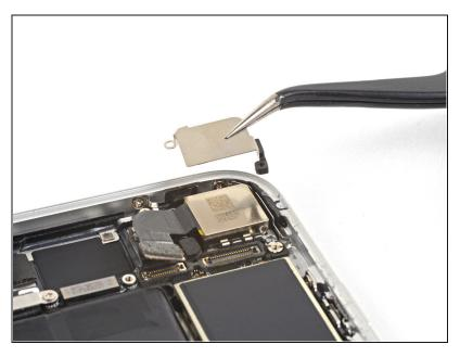
• Remove the rear-facing camera bracket.
