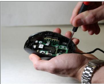
• Using the Phillips #00 screwdriver, unscrew the three internal screws.
