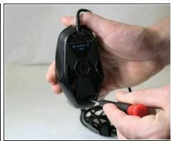
Using a Phillips #00 screwdriver, unscrew the three screws that hold the top and bottom halves
