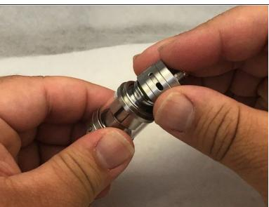
Remove the bottom lid from the tank. The bottom lid holds the coil inside the tank. By removing the bottom lid, you are able to take out the coil.
