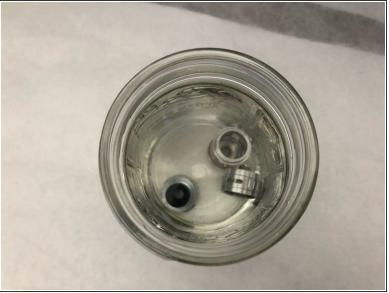
• To clean the tank and the lids, you need to submerge them in a glass of water for approximately 3-4 minutes to make sure they are cleaned properly.
