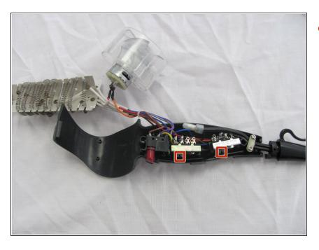
Locate the two switches in the handle of the device.
