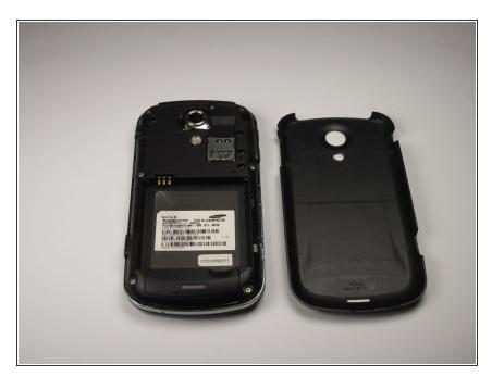
Remove the battery from the device by pulling the battery edge upwards.
