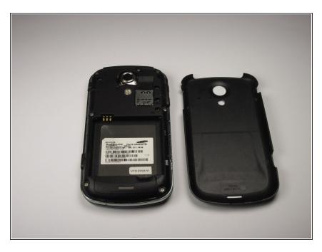
Pull at the plastic backing gently to remove it after hearing the snap sound.
