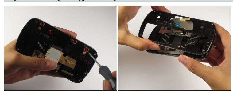
Remove the four Phillips #00 screws on the keypad housing.
