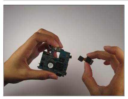
Remove and replace the camera lens with a new one from a manufacturer.
