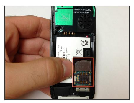
With the battery removed, locate the SIM card slot on the lower right side of the back of the phone. Gently slide the SIM card out from the slot.
