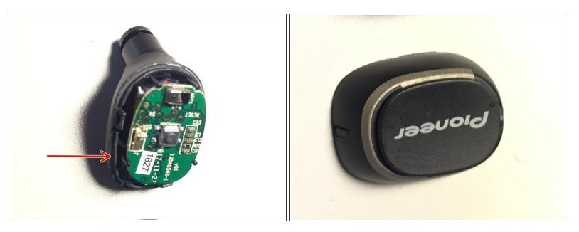
Apply a little bit of amount of Kola Loka (using the point of a needle) on the circumference of the earphone and glue them. apply force while it dry.
