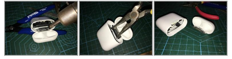
Heat with a hot air gun, cover the metal connection parts, the temperature here is slightly higher, about 90 to more than 100 degrees, after heating for 20 seconds.
