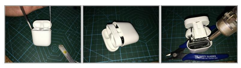
After loosening, use a metal lever, pull both sides at the same time, then pay attention to the cable to pull out the internal base and finally heat with a hot air gun to remove the stainless steel internal fixed iron ring.
