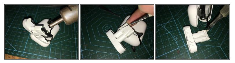
After heating the base of the contact, use a scalpel to open it. The adhering parts become loosened further so you can finally remove them from the bottom.
