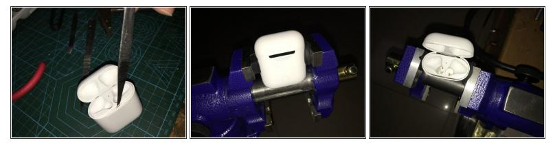
Use a polished metal lever to loosen it further, then fix it with a vise grip, tighten it slowly to deform the load and outer shell, and then loosen with the tool. (Remember to secure the AirPods on both sides of the shell before attaching it. Prevent the press from leaving traces on the outer casing.)
