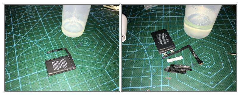
After removing the battery, remove the protective plate position, clean it with internal wash water and recharge it with an adjustable DC power supply.
