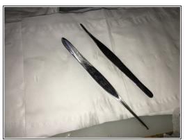
Find a pair of tweezer, and then divide it into two halves to create a spudger. Then grind it with a grinder to the size required to be reasonably long and thick, ready for the next step of disassembly! Or buy one from ifixit
