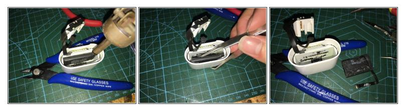
After continuing to heat with a heat gun, loosen the battery with a lever, loosen the push button on the base of the fixed connection cable and remove the battery.
