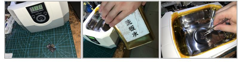
• First I use the ultrasonic cleaner with PCB cleaning liquid to try and save the circuit board.
