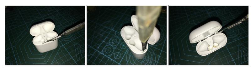
Using a scalpel, insert the inside and outside to slide left and right so that the connection parts of the charging case are completely loose, and then lift a space and insert a tool as a lever.
