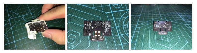
After pulling away the circuit board, you can see that some of its components are very corroded.
