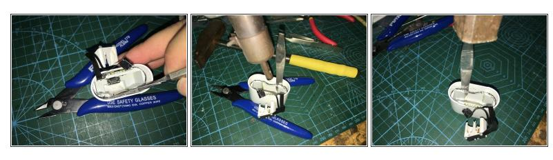
• Use the scalpel to slide the inner frame and fixed frame to the left and right to loosen the attachment parts. You can use the heating method to slide while heating, and then use the special metal lever polished before the hammer to force down.
