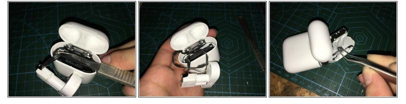
After removing the stainless steel fixed iron ring, then use a heat gun to heat, the indicator light and the charging contact base of the AirPods.
