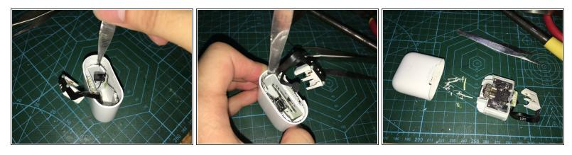
Continue repeating the previous operation until it is completely loose, and finally remove the internal support.
