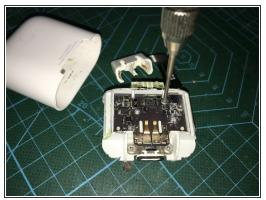
After complete removal, remove it with a screwdriver and connect the cable at the base of the headset to the cable that is loaded with the lightning interface below.
