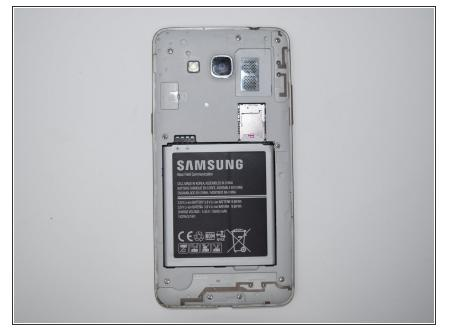
Insert the new battery in the reverse order from taking out the battery, ensuring the metal contacts from the phone are touching the flat metal contacts on the battery. Then place another edge of battery in the bay.
