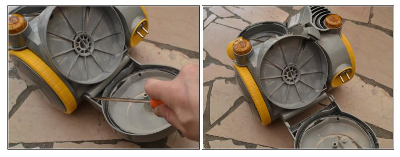
Optionally, remove the rear filter cover.
