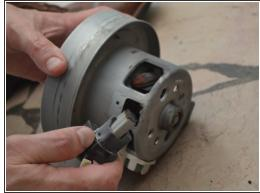
disassembly of 2 engine coals (1 Phillips screw per coal)
