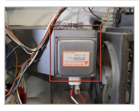
Sparking inside of the microwave may also be the result of a broken or misaligned magnetron. If this is the case, it is recommended to take the microwave to a qualified professional or completely discarding the unit and purchasing a new one.
