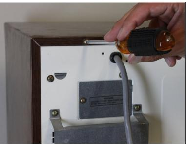
Remove the additional four screws securing the wood-paneled case to the microwave frame.
