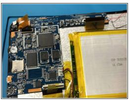
Next using the flat end of a plastic spudger release the clips holding the ribbon circled in the first picture.
