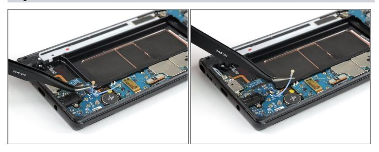
• Use a pair of tweezers to carefully disconnect both ends of the blue coax cable and remove it.
