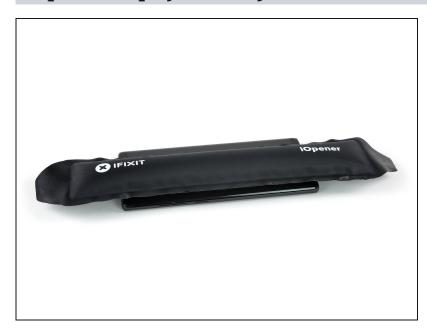
Prepare an iOpener and apply it across the phone to loosen the adhesive beneath the vibration motor at the bottom and the earpiece speaker at the top.
