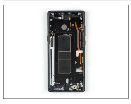
To reassemble your phone transfer all components you removed to the new display assembly with frame. Reapply adhesive where it's necessary. If possible, turn on your phone and test your repair before installing new adhesive and resealing the phone.
