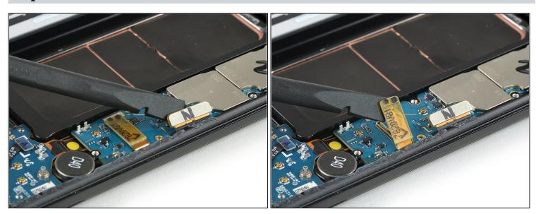
• Use the flat end of a spudger to disconnect both the display and the touchscreen cables.
