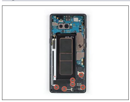
Remove the six Phillips #00 screws on the loudspeaker assembly at the bottom of the phone.
