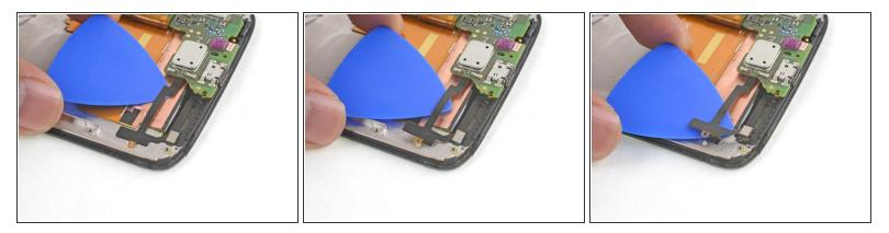
Insert an opening pick underneath the flat flex cable and slide it to free the cable from the frame.
