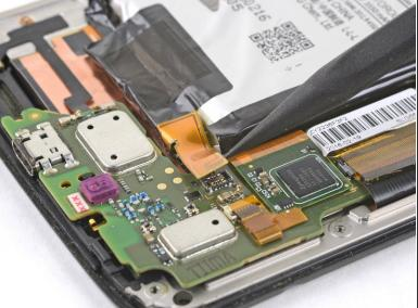
• Use the point of a spudger to pry up and disconnect the battery pack connector.
