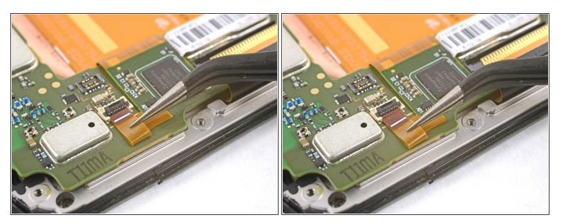
Use tweezers or a spudger to walk the ribbon cable out of the ZIF connector.
