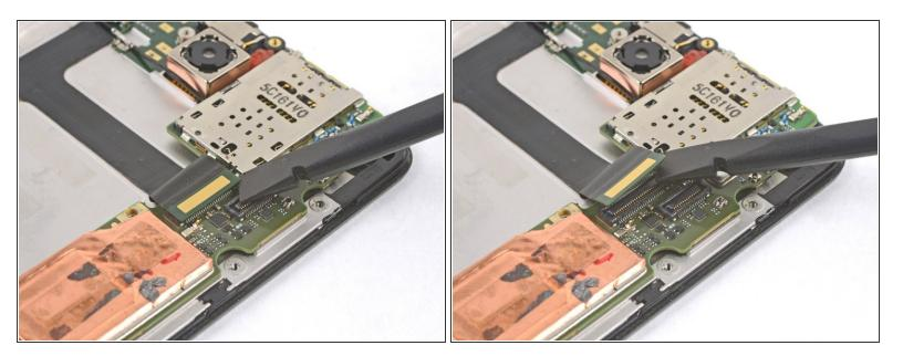
Use the flat end of a spudger to pry up and disconnect the accessory module connector.
