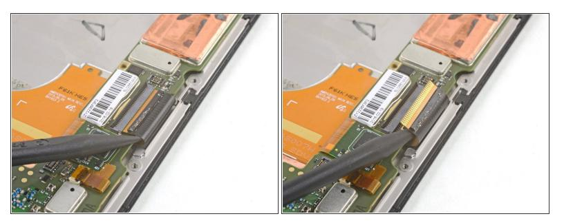
Use a spudger or tweezers to walk the flat cable out of the ZIF connector.
