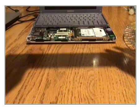
Re-connect the ribbon cable from the trackpad/wrist-rest, then place the assembly down onto it's mount and close the computer lid, and then flip it back over.
