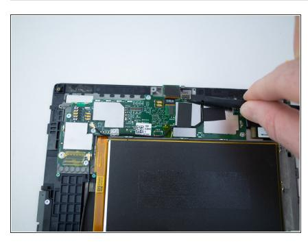
Use the flat end of a spudger to disconnect the front camera press-fit connector from the motherboard.
