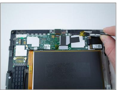
Grab the yellow tape with a pair of tweezers and pull upwards to disconnect the press-fit connector.
