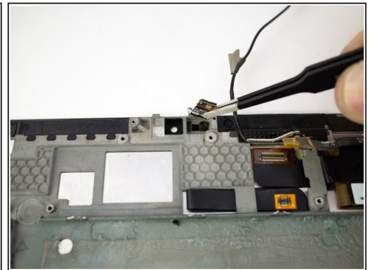
**i** The motherboard has been removed in this image, but its removal is not necessary to complete this replacement.
