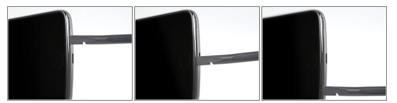
Insert the flat end of a spudger into the seam and slide it along the bottom edge to release the clips holding the back cover to the phone.
