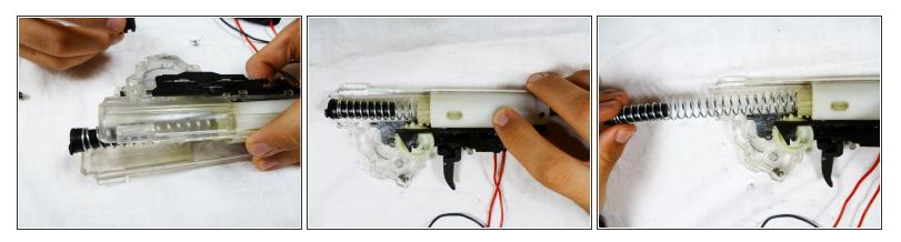
• Remove the cover and pull out the spring.
