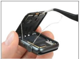
↑ To avoid straining the display cables, don't open the display all the way yet.
