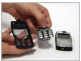
After removing the front cover, simply peel the keypad away from the front cover
