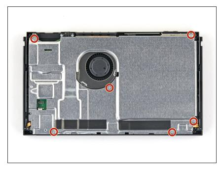
Use a JIS 000 screwdriver or an official iFixit PH 000 driver to remove the six 3 mm screws securing the shield plate to the device.
