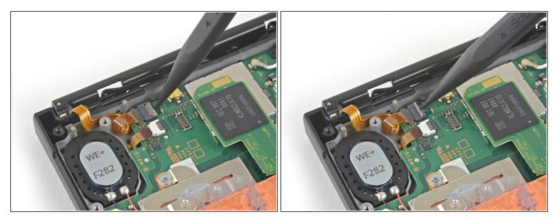
Use a spudger, opening tool, or your fingernail to flip up the small, hinged locking flap on the Joy Con rail data cable's <u>ZIF connector</u>.
