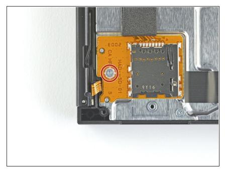
Use a JIS 000 screwdriver or an official iFixit PH 000 driver to remove the 3.1 mm screw securing the microSD card reader to the device.
