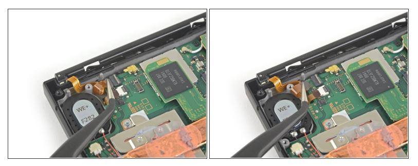
• Use a pair of tweezers to slide the Joy Con rail data cable out of its connector on the motherboard.
