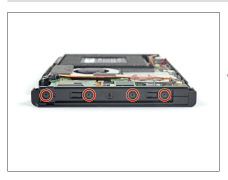
Use a JIS 000 screwdriver or an official iFixit PH 000 driver to remove the four 3.7 mm screws securing the
