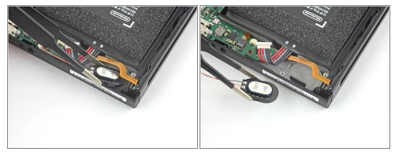
• Use your fingers or a pair of tweezers to carefully remove the speaker from the speaker well.
