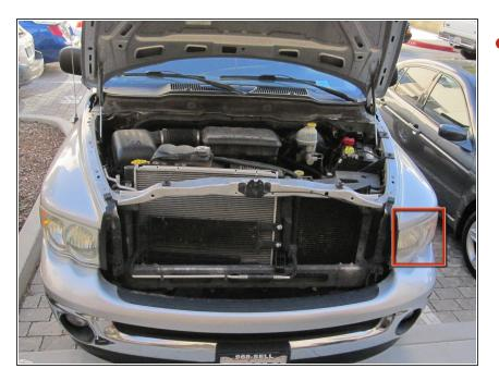
In this guide we will be removing the left headlight. The steps are mirrored for the right headlight.
