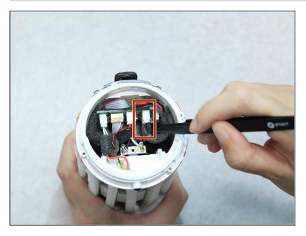
• Use the angled <u>tweezers</u> to disconnect the battery from the motherboard. It will take some work to remove this piece.
