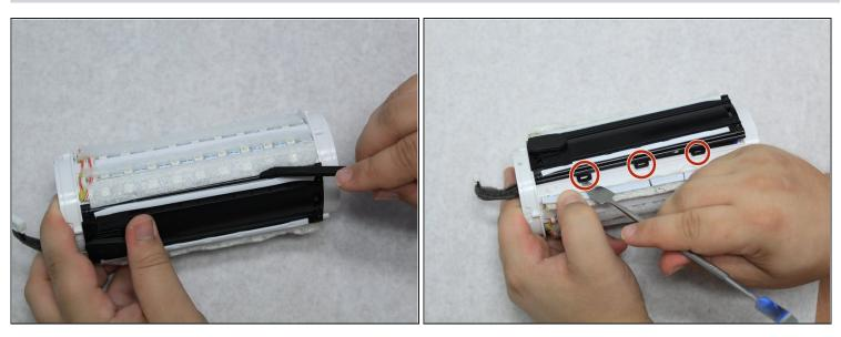
• Use the spudger to reach under the sides of the black centerpiece to access the six latches, three of which are on each side.
