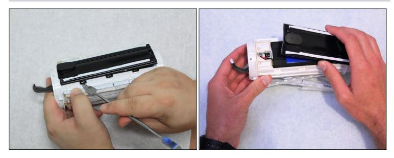
• Lift the black centerpiece off with the metal spudger to reveal the battery underneath.
