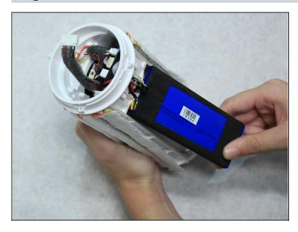
• Use a hot air gun to soften the hot glue in order to fully remove the battery.
